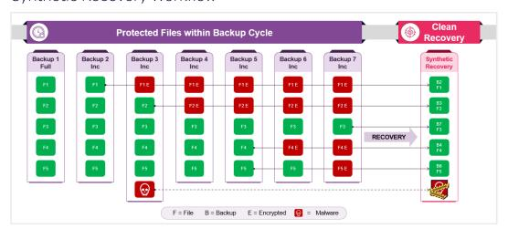
The diagram to the left visually demonstrates how Synthetic Recovery assembles clean data from multiple backups while quarantining malware and infected versions. Visual of how Synthetic Recovery pinpoints and removes compromised data (patent-pending).
