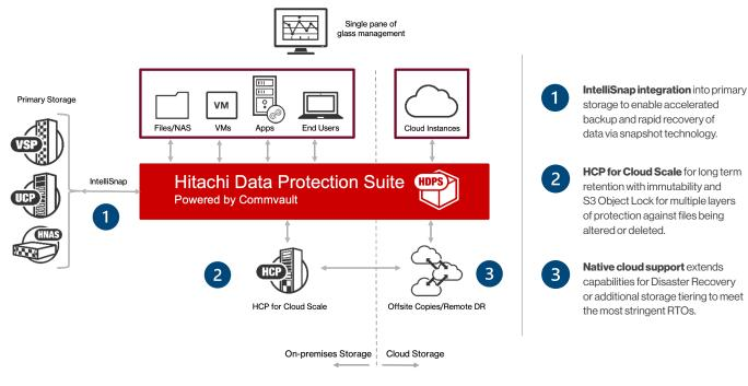
Fig. 5 Complete Ransomware Protection with HDPS and HCP
